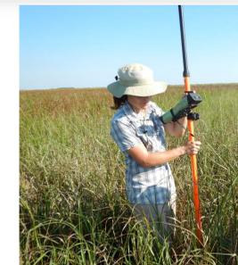
Fig. 9. Taking elevation measurements with Leica RTK GPS in created marsh
